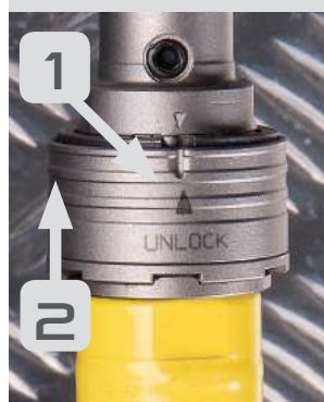
RELEASING A HOLE SAW
