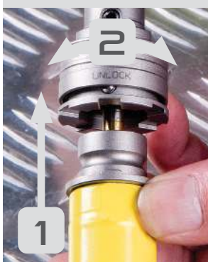
ATTACHING A HOLE SAW
